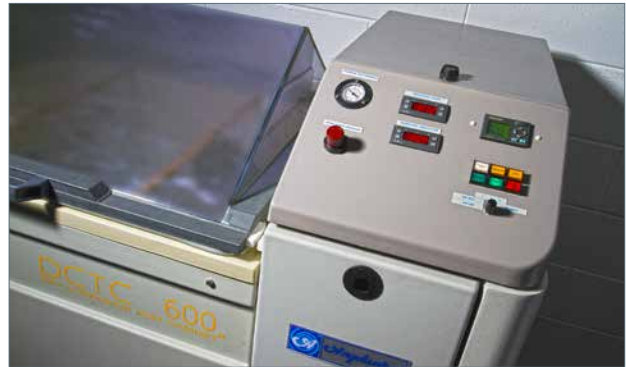
Salt spray testing equipment.
