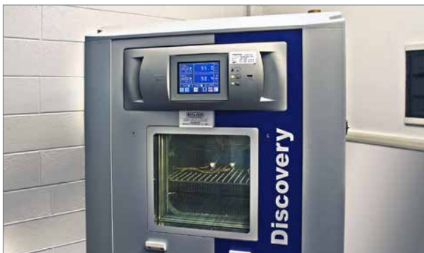
Discovery climatic chamber testing equipment.
